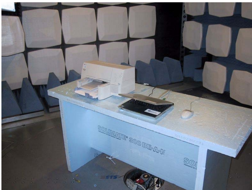
Picture 2: Radiated emission measurement setup
