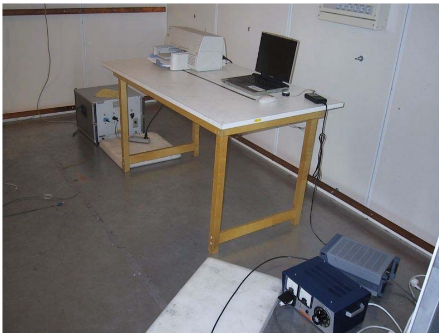
Picture 3: Conducted emission measurement setup
