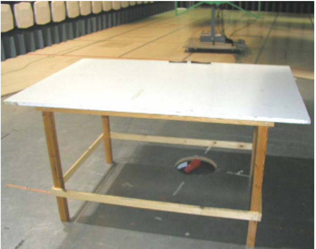
Photograph 1. Radiated emissions test setup
