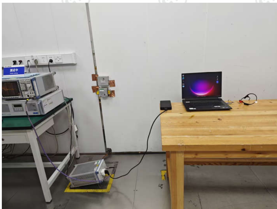
Conducted Emissions Test Setup
