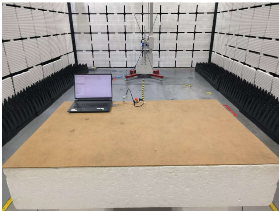
Radiated spurious emission Test Setup-1(Below 1GHz)
