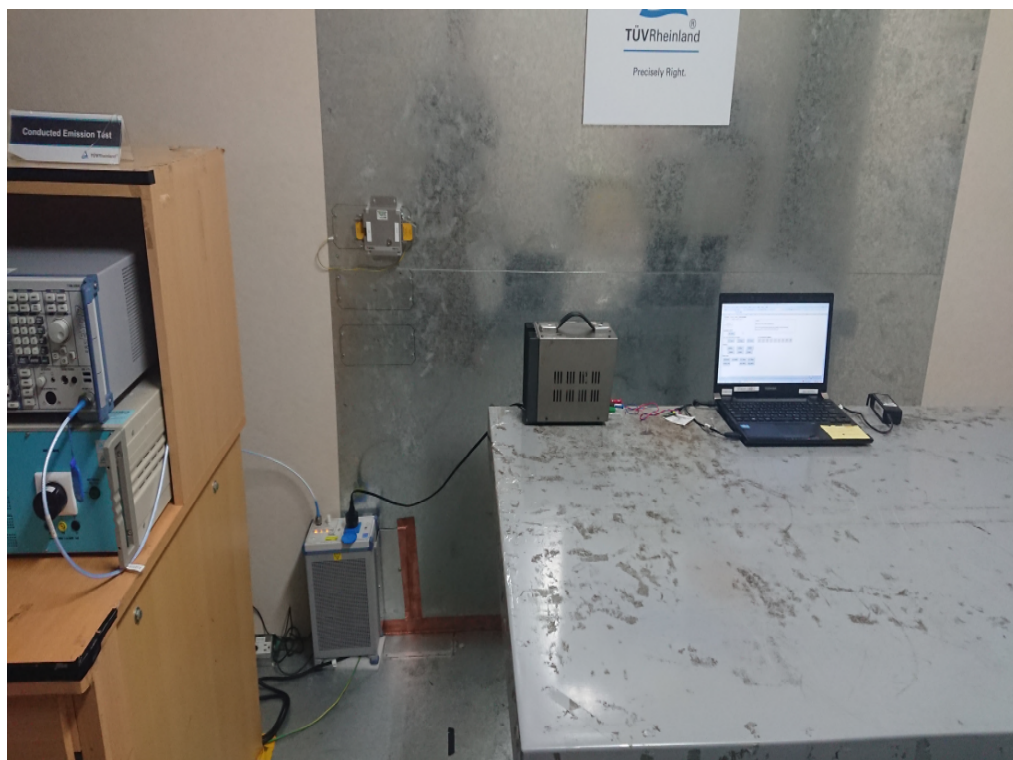
Photograph 7: Set-up for Mains Conducted testing (Front View)
