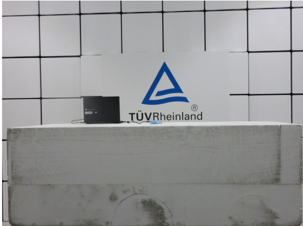
Photograph 3: Set-up for Spurious Emissions (Back View 1)
