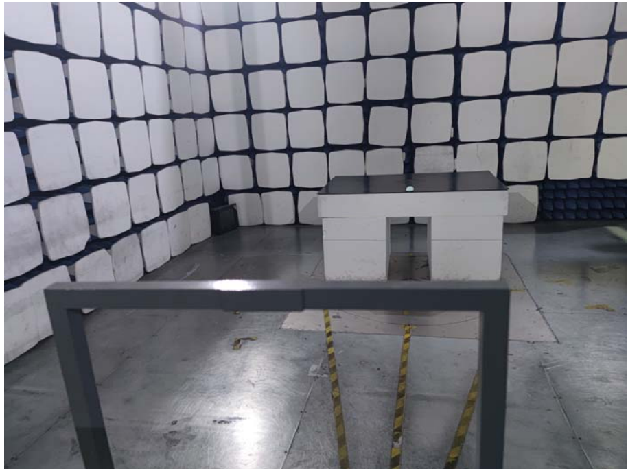
Radiation Emission Test Setup (Below 30MHz)
