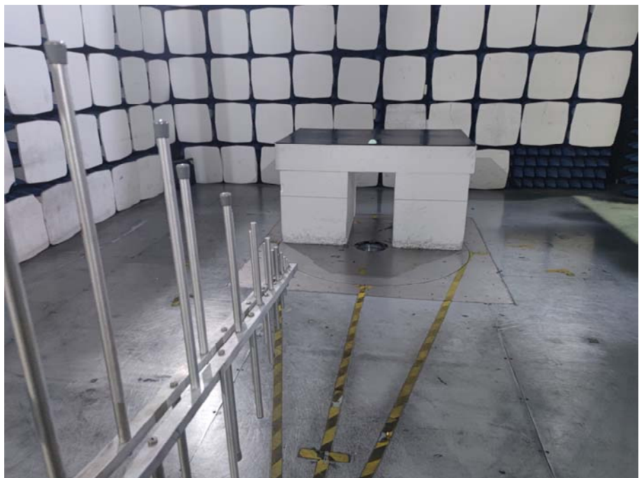
Radiation Emission Test Setup (30MHz to 1GHz)
