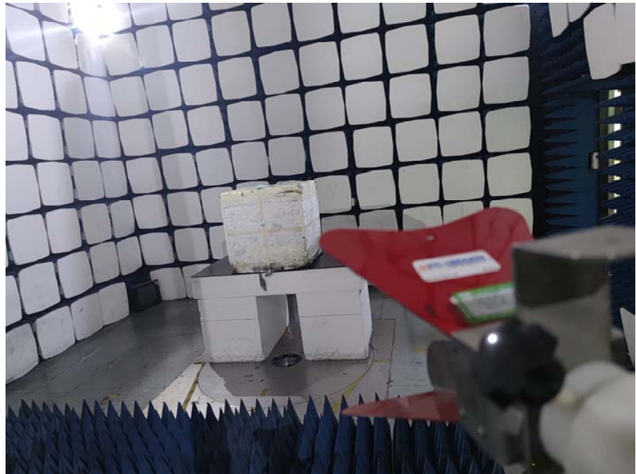
Radiation Emission Test Setup (1GHz to 18GHz)
