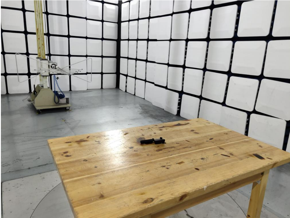
FCC ID: RZO-TP-RGH10 Photo of Radiation Emission Test
