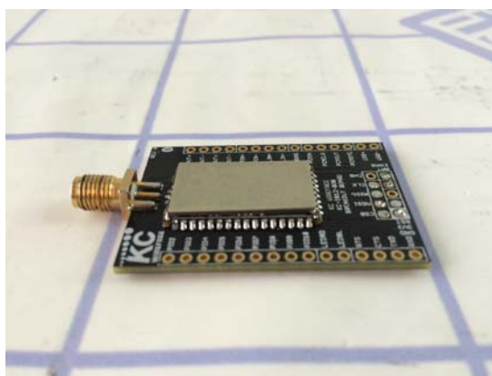
External Antenna type External view-5
