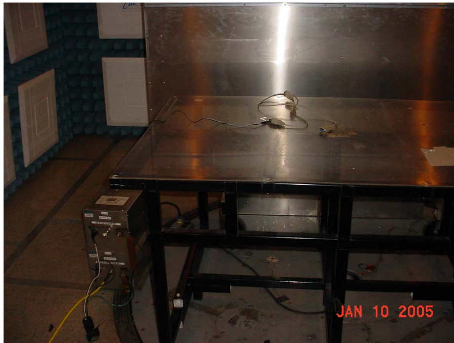
Figure 2 - Powerline Conducted Emissions 150kHz – 30MHz
