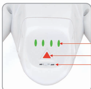
2.4 Turn the power switch to "ON" position, and press on the power button about 3-5 second till the green LED light solid. The undercarriage(skid landing) will unfold automatically.
