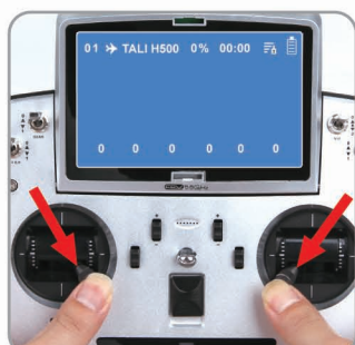
3.1 Enter into Compass Calibration, Aircraft red, green LED light flash quickly.
