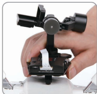
4.3 Put the Gimbal sliding chute aim to gimbal fixed block, and enclose to the bottom of gimbal fixed block.
