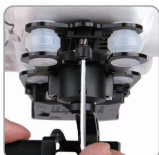
4.4 Put the spring into M3x12 screw, aim to the threaded hole, tighten up the screw to Gimbal.
