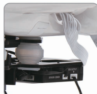
5.4 Insert the camera power cable into power output port of G-3D.
