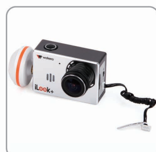
5.1 Screw the camera mushroom antenna into Camera.
