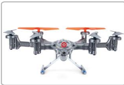
Chart 4: The red indicator light solid means calibration is successfully, and then put the aircraft at horizontal place.
