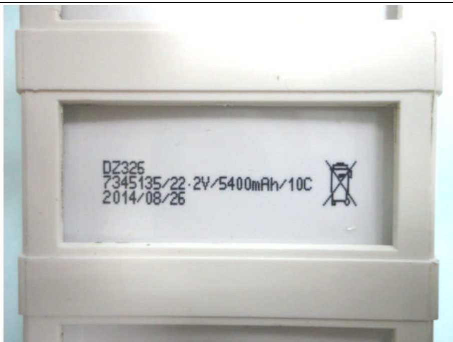
Picture 8: Battery pack
