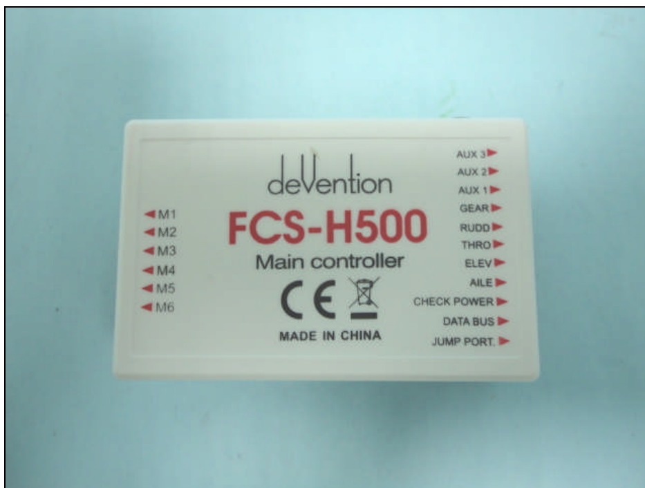
Main Controller Module
