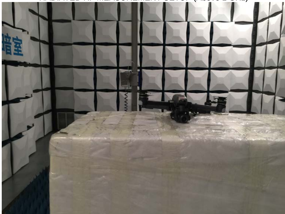
RADIATED RF MEASUREMENT SETUP (Above 1 GHz)
