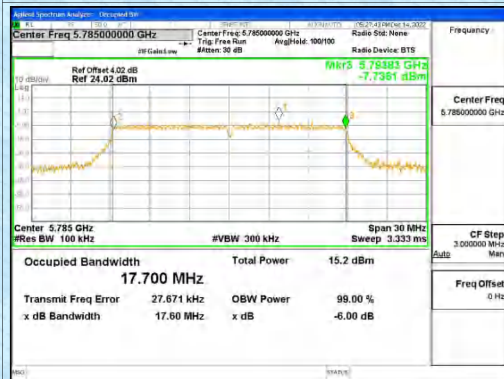
-6dB Bandwidth NVNT n20 5825MHz Ant1
