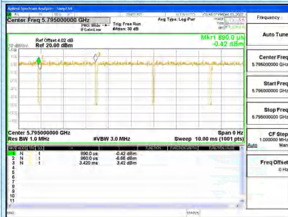
Duty Cycle NVNT n40 5795MHz Ant1
