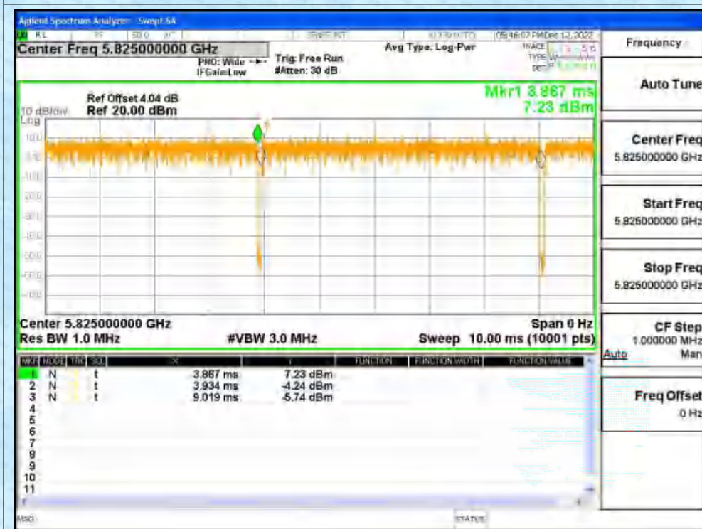
Duty Cycle NVNT n20 5825MHz Ant1
