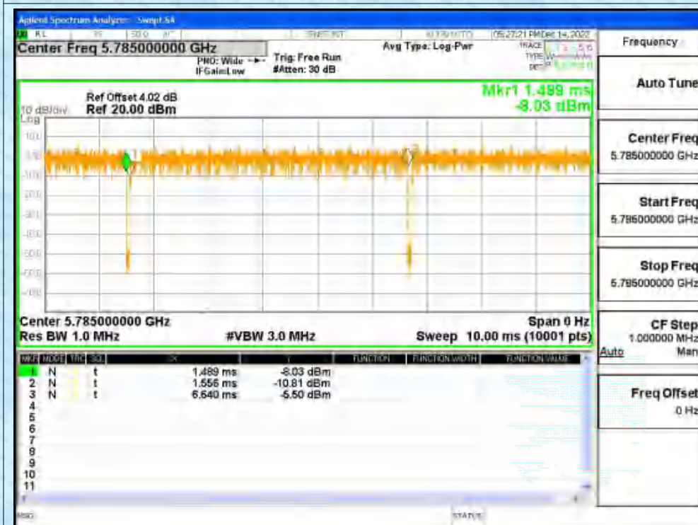
Duty Cycle NVNT n20 5825MHz Ant1
