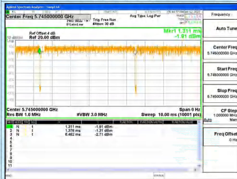
Duty Cycle NVNT n20 5745MHz Ant1
