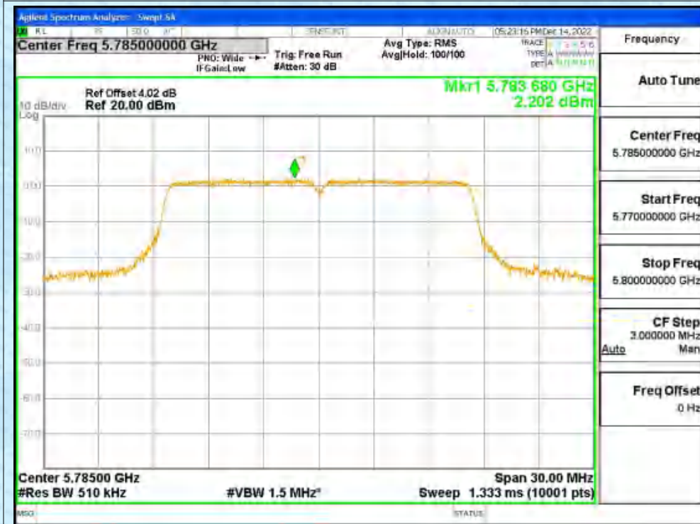
PSD NVNT a 5785MHz Ant1
