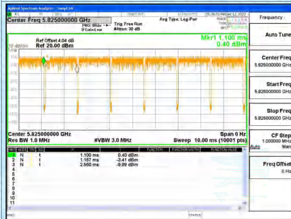
Duty Cycle NVNT n20 5745MHz Ant1
