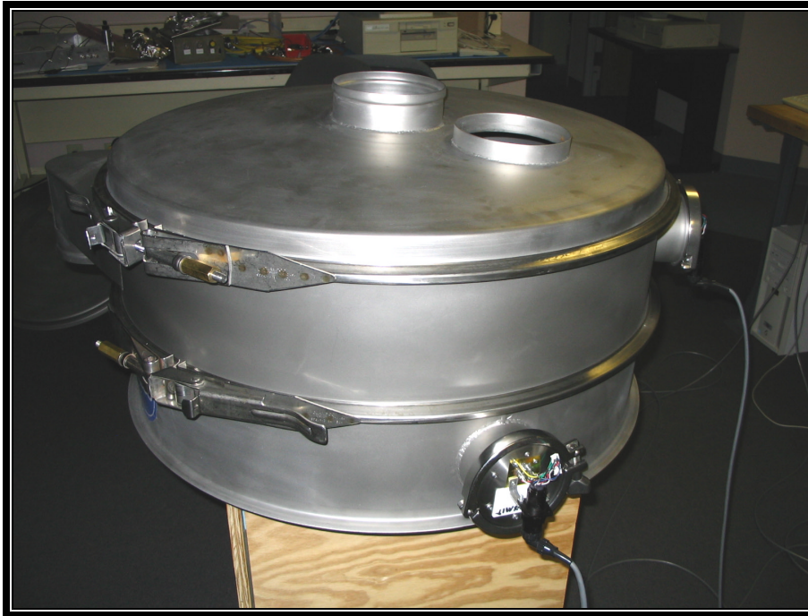
PHOTOGRAPH 9: VIEW OF TRANSMITTER AND RECEIVER WITH CABLES
