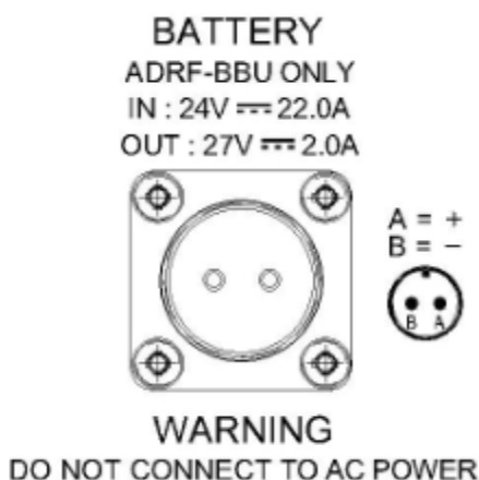
Figure 2-5 Battery Backup Port
