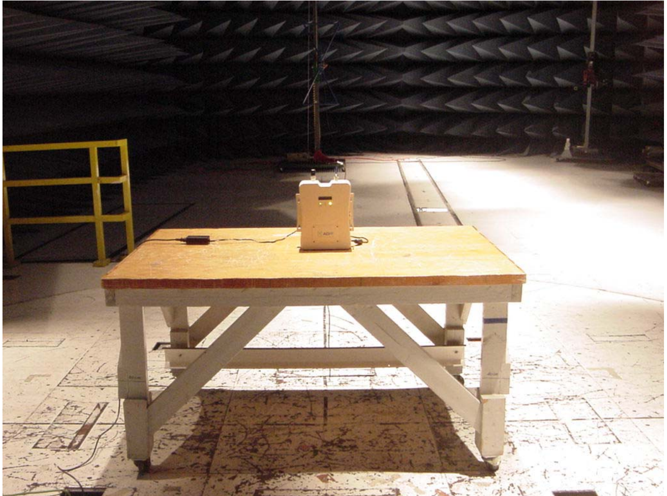
Photograph 3. Radiated Emission Limits Test Setup
