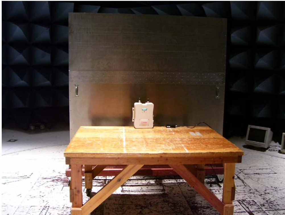
Photograph 2. Conducted Emissions Test Setup, Front View
