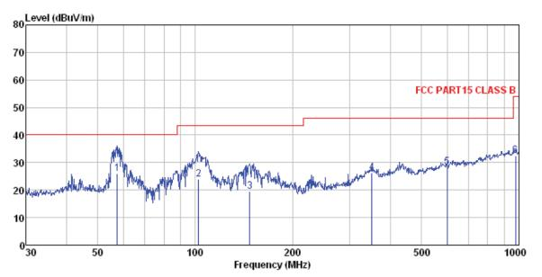
Site Condition : 3m chamber : FCC PART15 CLASS B 3m VULB9163-2013M HORIZONTAL
