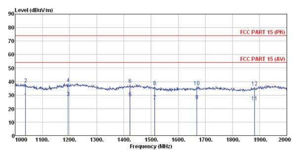
: 3m chamber : FCC PART 15 (PK) 3m BBHA9120D ANT(>1GHZ) VERTICAL : 1212RF Condition
