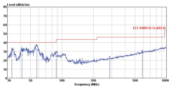
Site Condition : 3m chamber : FCC PART15 CLASS B 3m VULB9163-2013M VERTICAL
