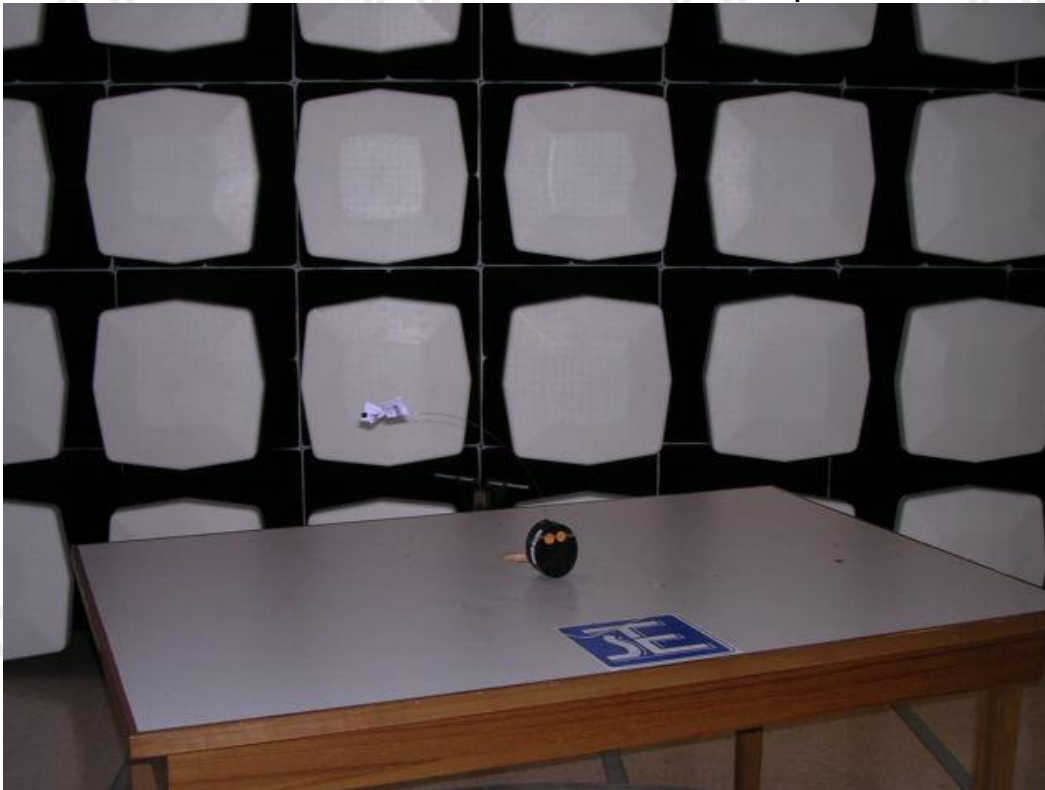
Measurement of Radiated Emission Test Set Up
