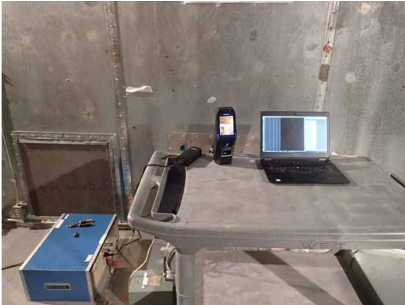
Power Line Conducted Emissions (EUT Powered by PoE Injector Power over Ethernet)
