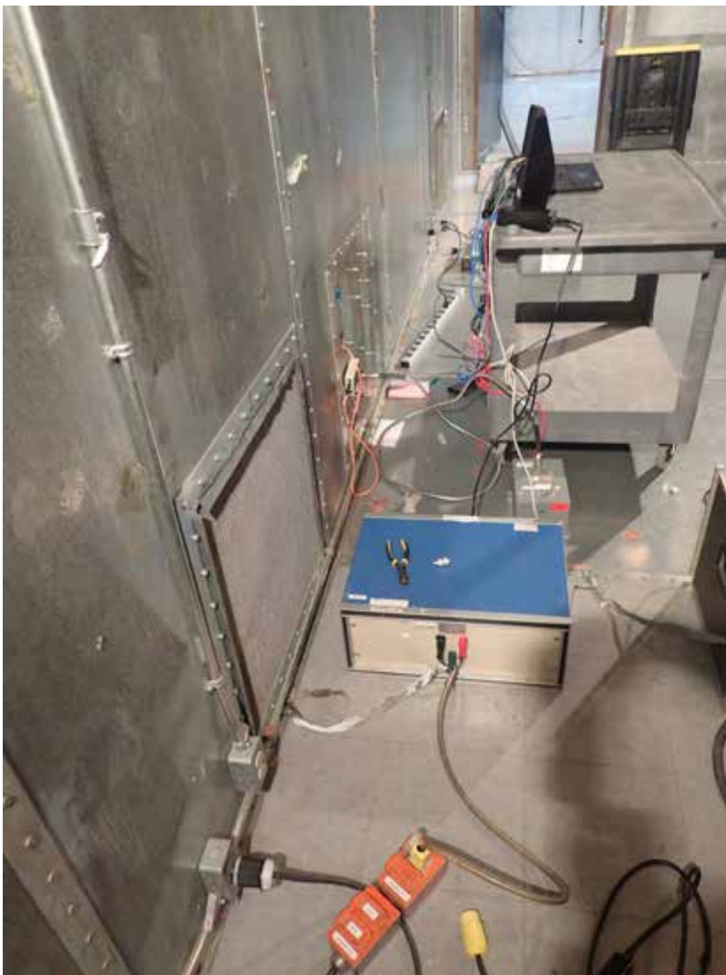
Power Line Conducted Emissions (EUT Powered by PoE Injector Power over Ethernet)
