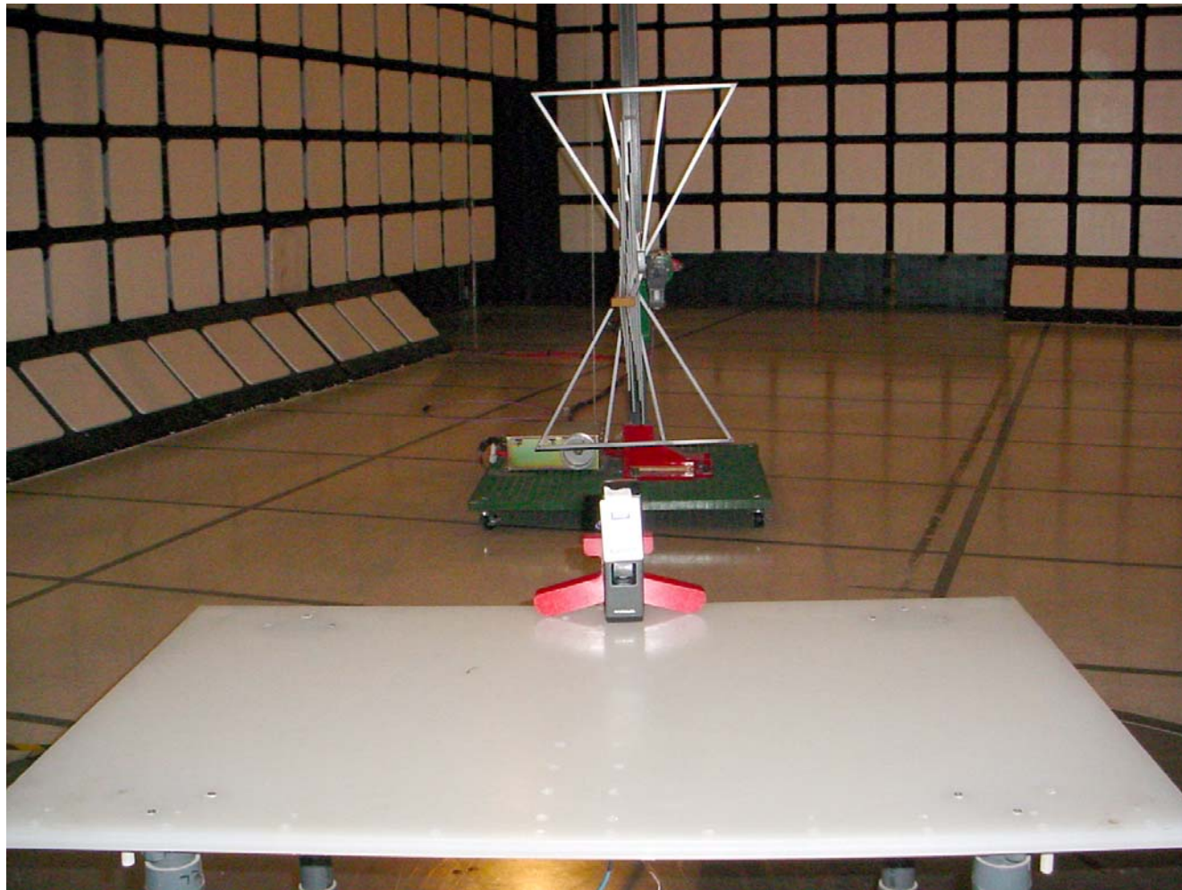
Radiated Emissions at 3 m Distance (30 MHz to 1000 MHz)
