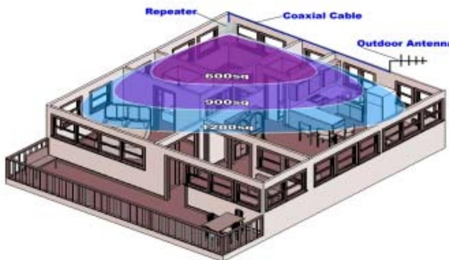
Figure 1: Typical Repeater/Coverage Configuration
