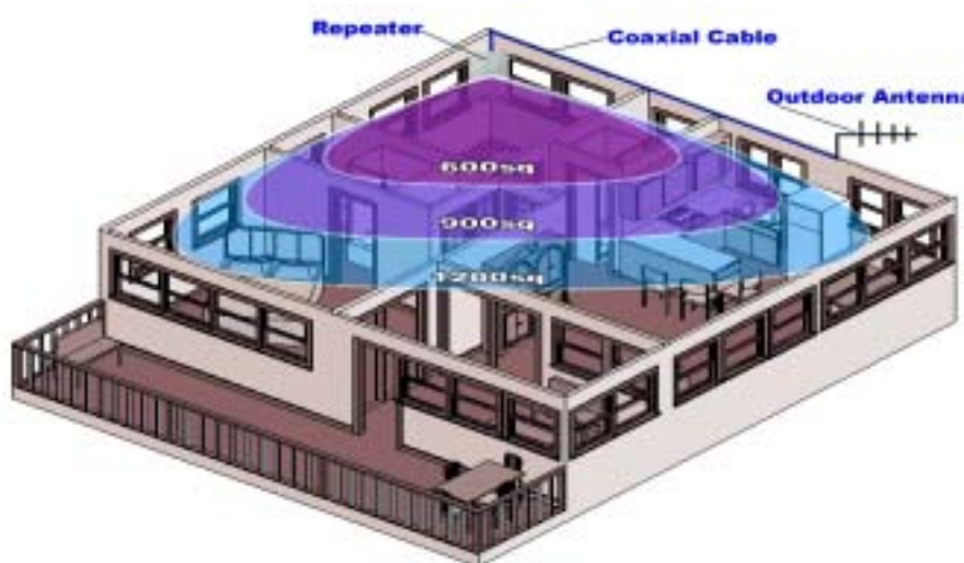
Figure 1: Typical Repeater/Coverage Configuration
