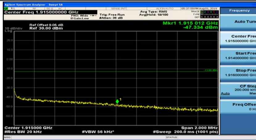
(Channel Bandwidth:20 MHz)_HCH_QPSK_1RB#49
