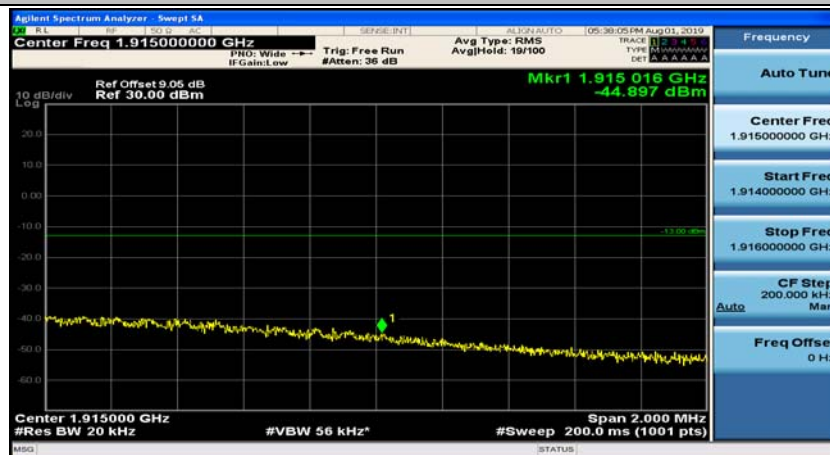
(Channel Bandwidth:20 MHz)_HCH_QPSK_1RB#99
