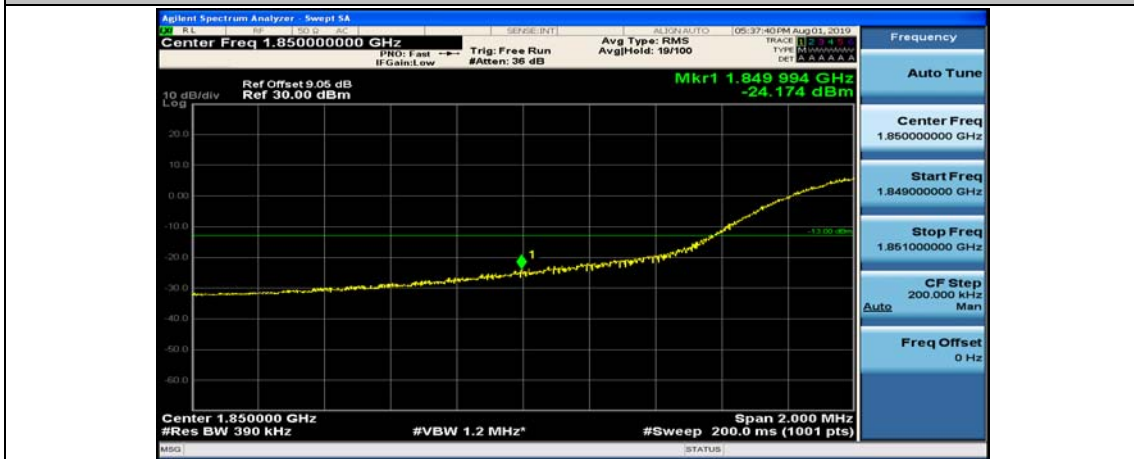
(Channel Bandwidth:20 MHz)_LCH_QPSK_100RB#0
