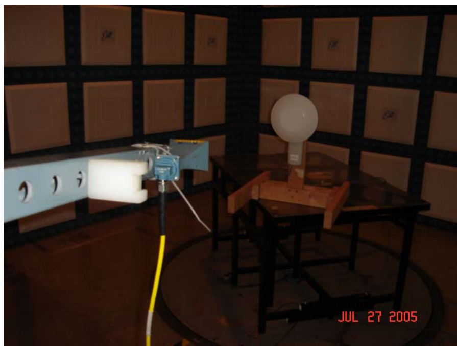
Test Setup for Measurement of Radiated Emissions
