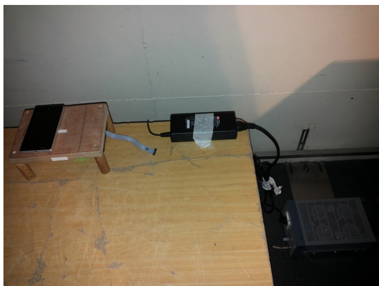
Photograph 7.2.3 Setup for conducted emission measurements, QI 5 Watt mode
