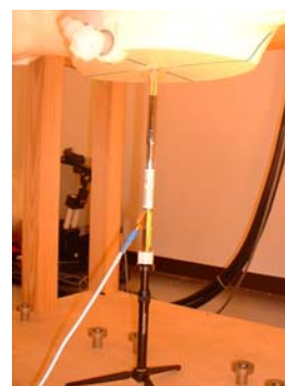
2450MHz System performance check setup
