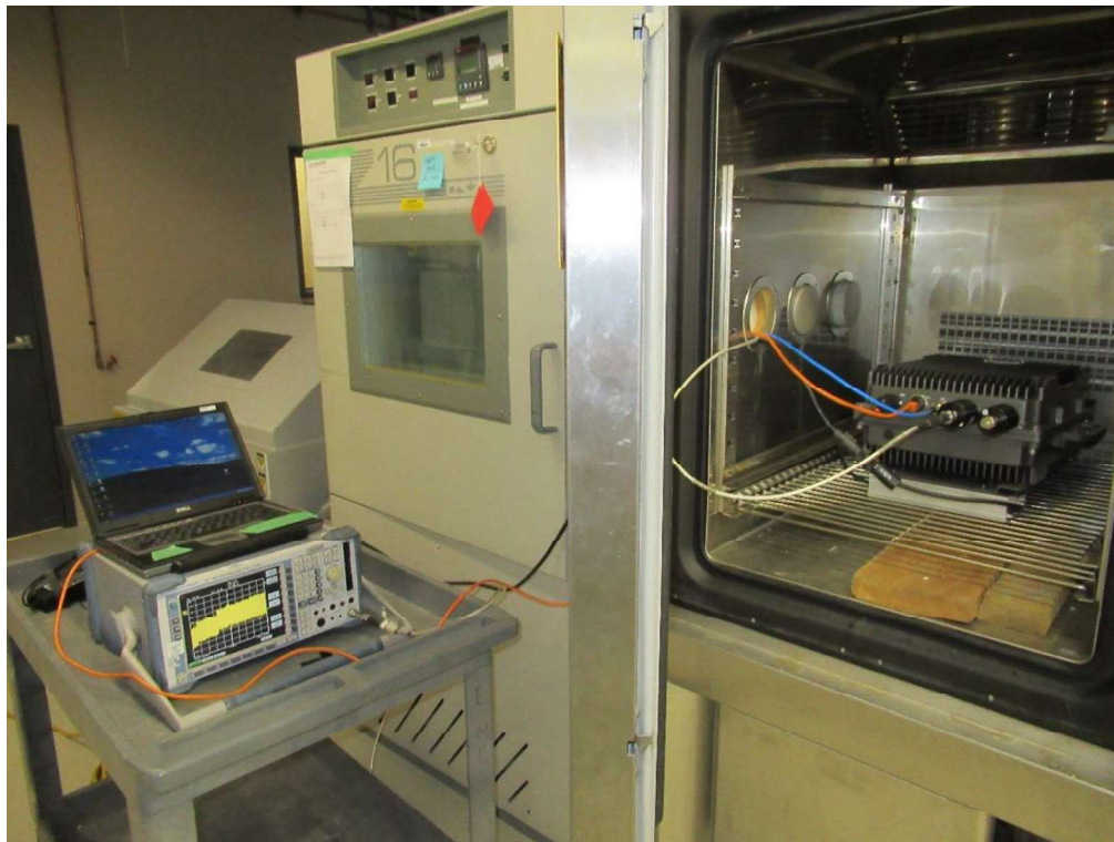
Figure 169: Frequency stability with respect to temperature test setup
