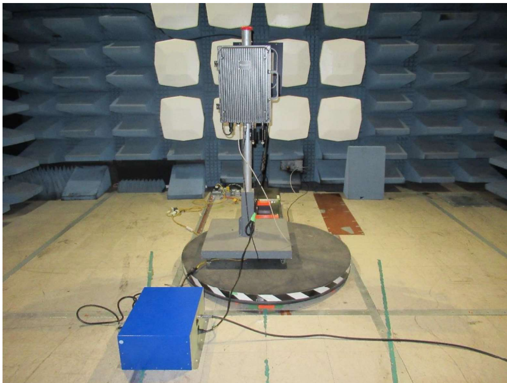
Figure 164: Radiated Emissions: 30 MHz – 1 GHz Measurement Setup
