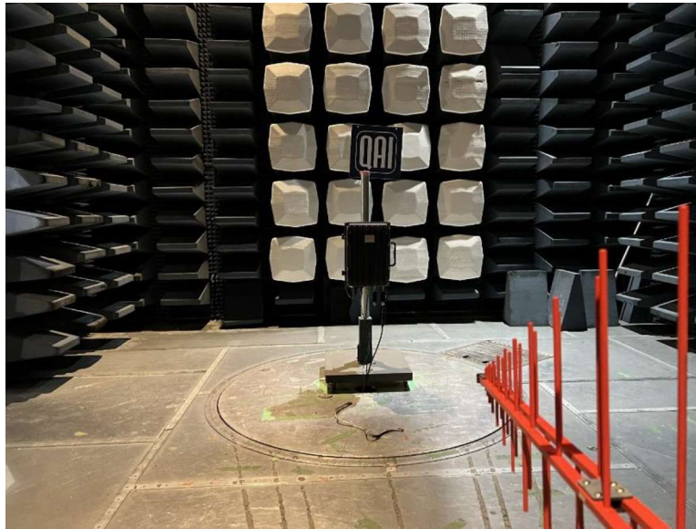
Figure 1: Radiated Emissions 30MHz– 1GHz
