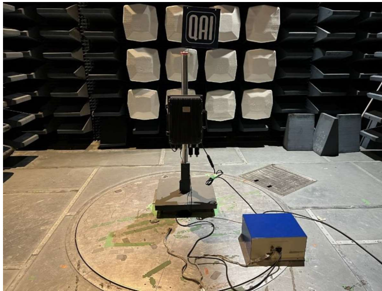
Figure 3: Conducted Emissions AC Main.
