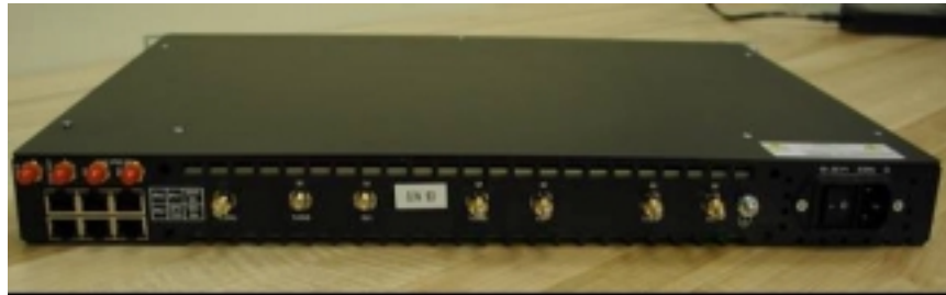
Figure 3-1: BTS 19' Rack Mont Rear View
