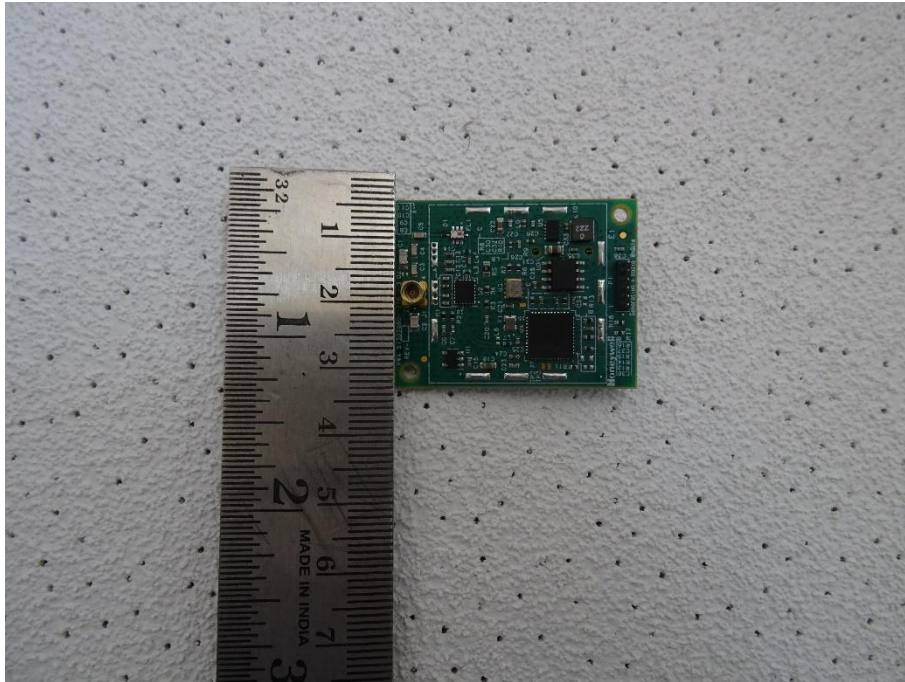
Photo 1: RF Module front and dimensional view
