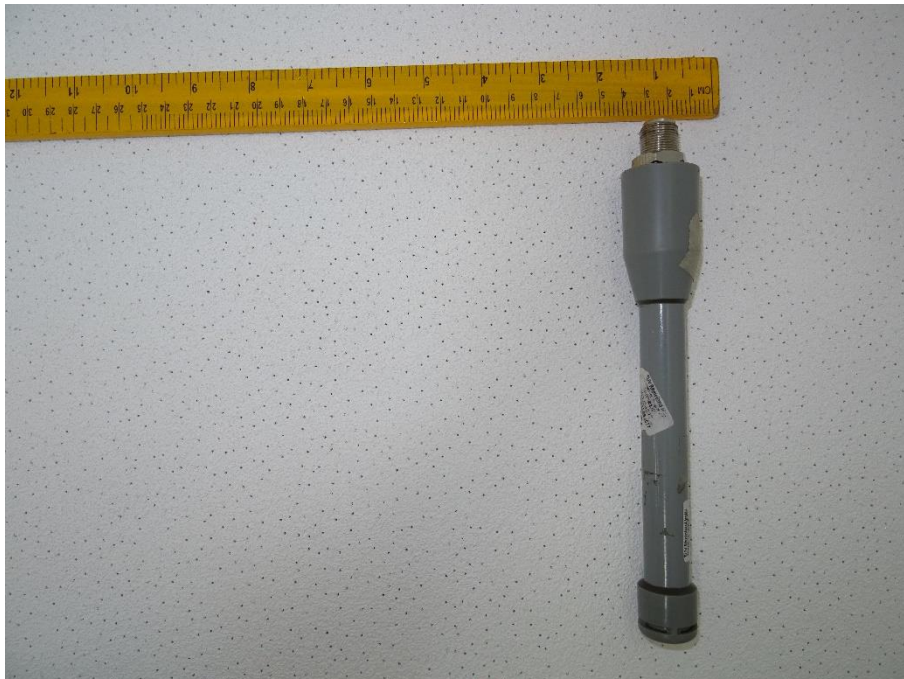
Antenna 4: HGV- 2404U antenna (4 dBi)
