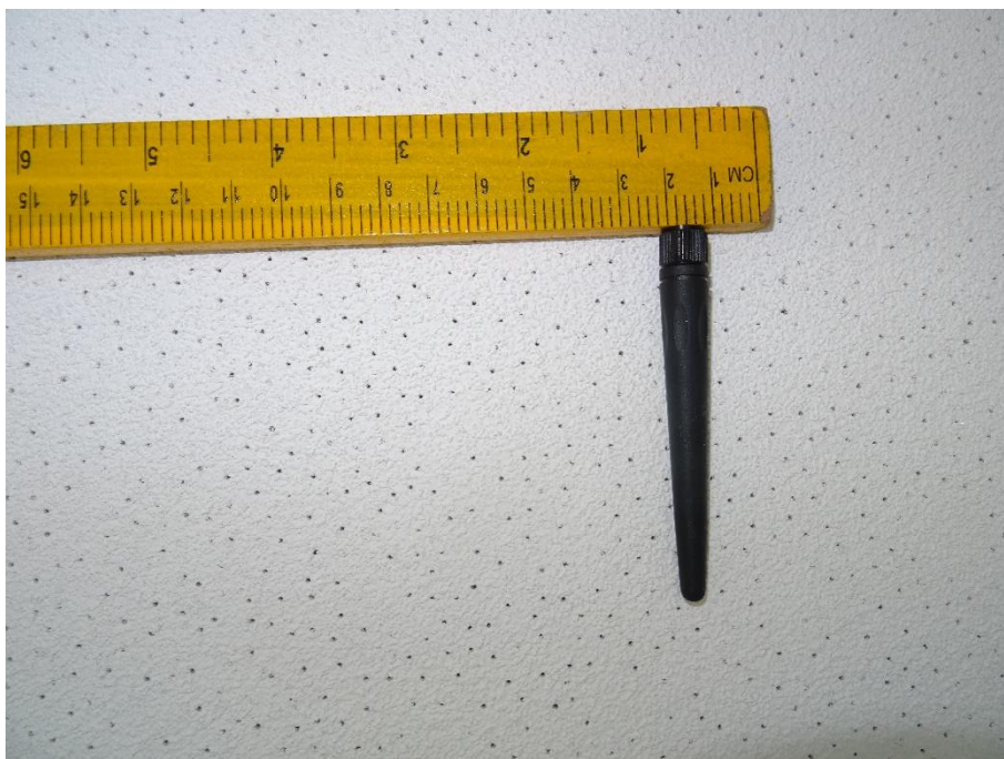
Antenna 2: HG2402RDR-RSP / Rubber Duck Omni antenna (2 dBi)
