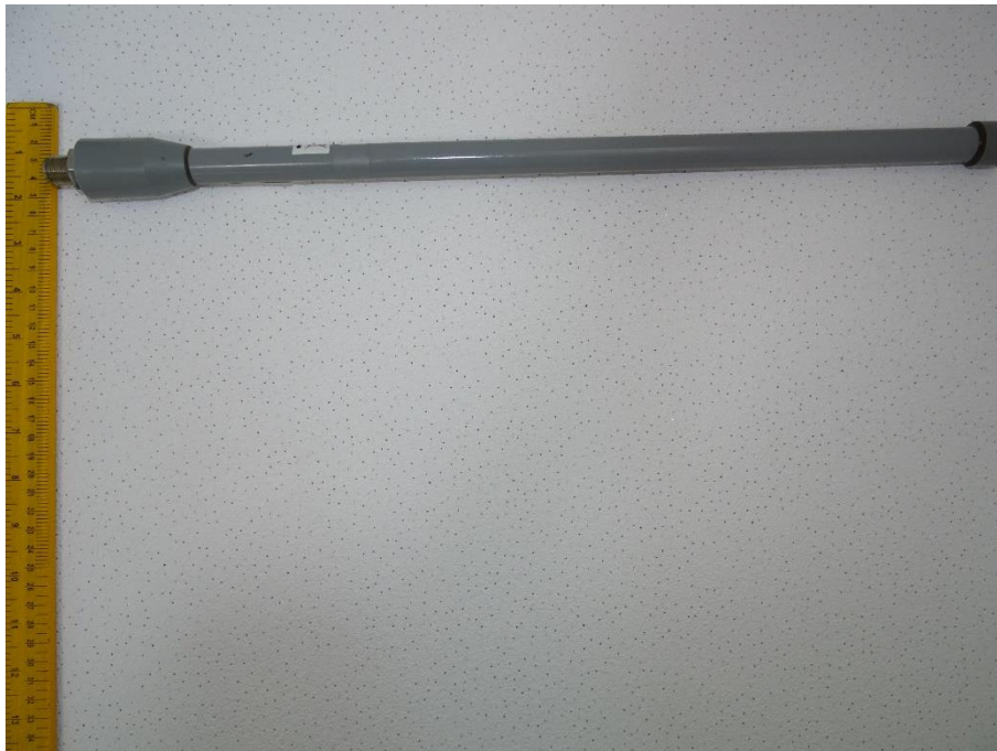
Antenna 5: HGV – 2409 U Omni antenna ( 8 dBi)
