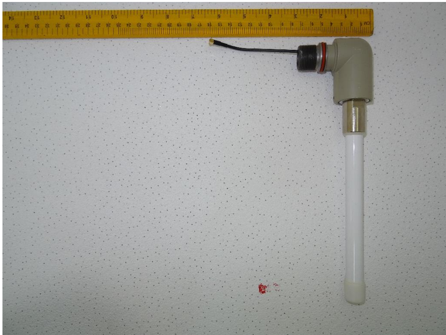
Antenna 3: EM-B14503-MMP-Z6 antenna (4 dBi)
