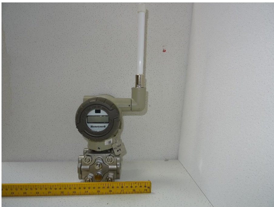
Photo 10: Dimensional view of Host with 4 dBi antenna
