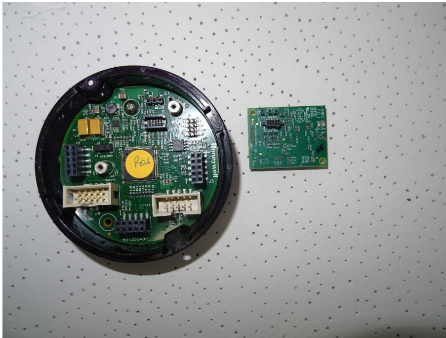
Photo 3: RF module removed from Host device
