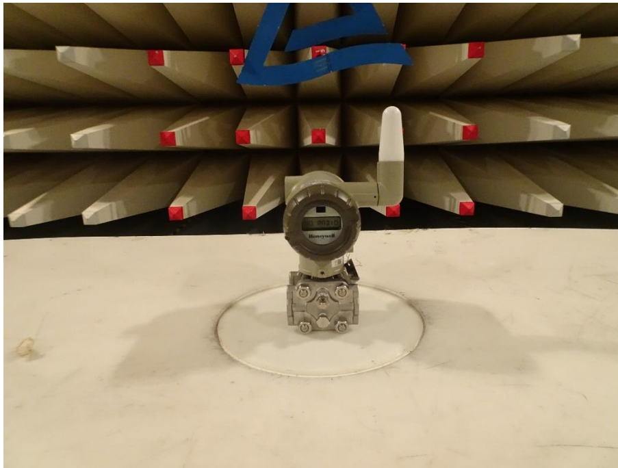
Photo 7: Host device on turn table for below 1000 MHz.
