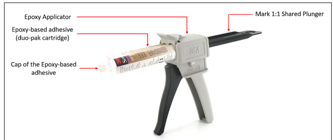
Figure 5-4: Epoxy Applicator loaded with Epoxy-Based Adhesive
