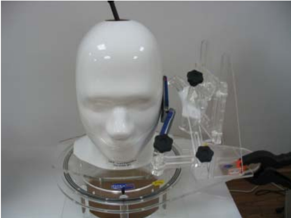
Fig.3 EUT Left Head Touch Cheek Position
