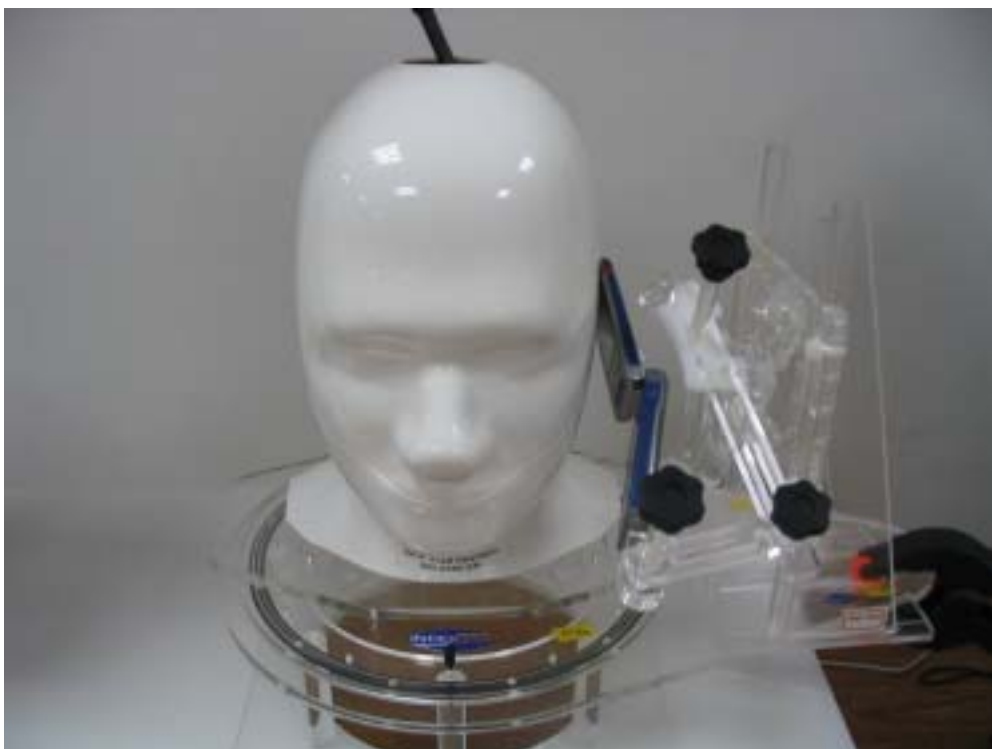
Fig.4 EUT Left Head Tilt15 Position
