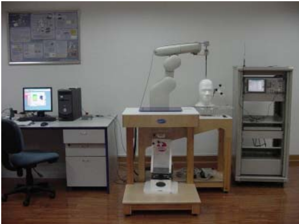
Fig.1 SARA2 System Test Layout
