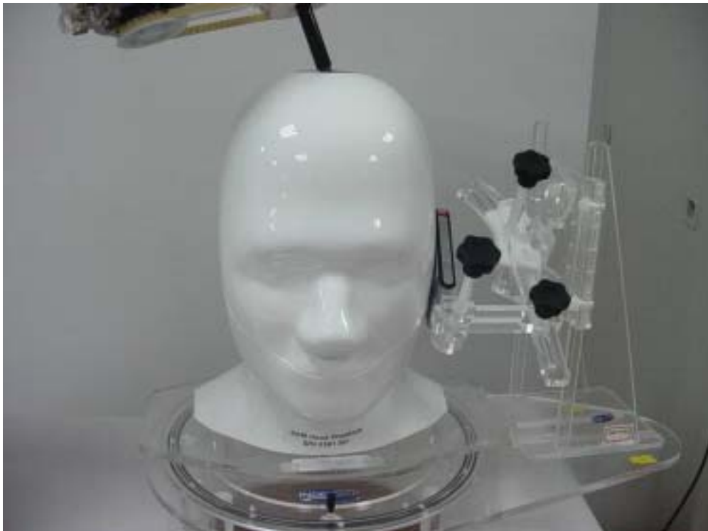
Fig.3 EUT Left Head Touch Cheek Position
