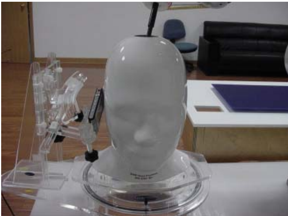
Fig.6 EUT Right Head Tilt15 Position
