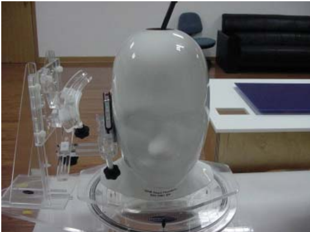
Fig.5 EUT Right Head Touch Cheek Position
