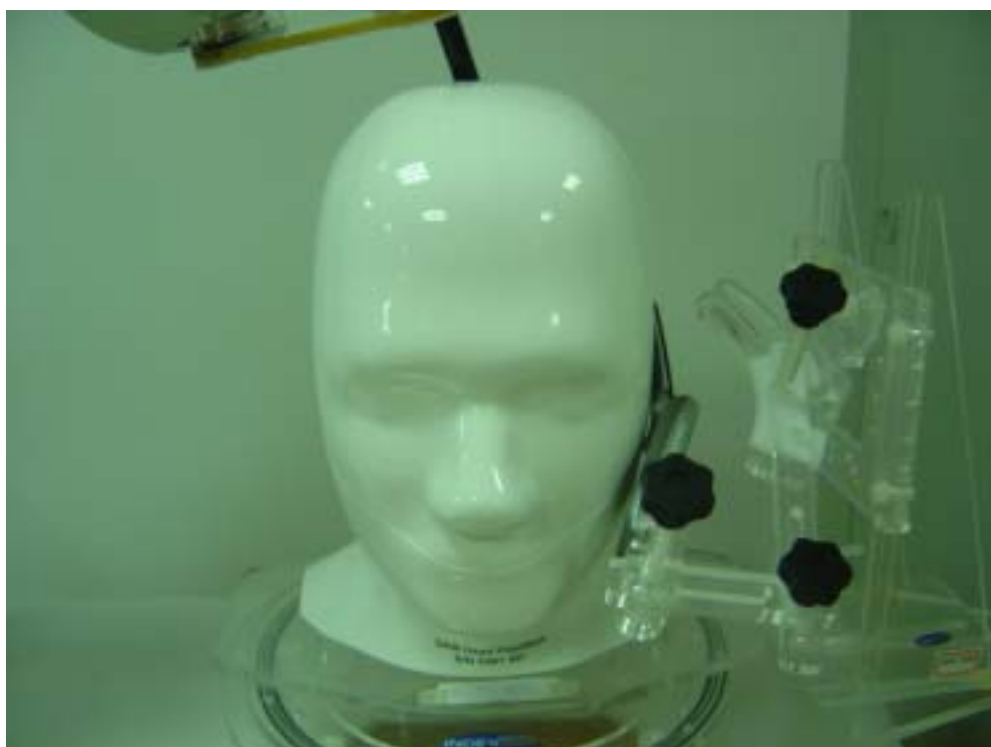
Fig.3 EUT Left Head Touch Cheek Position
