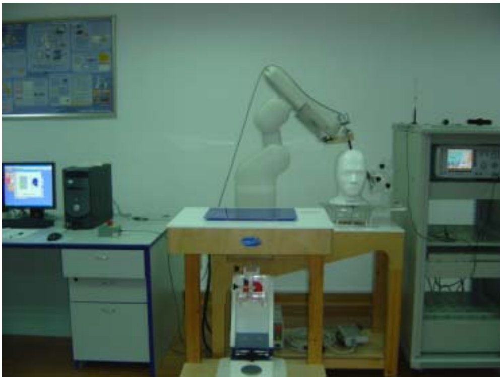
Fig.1 SARA2 System Test Layout
