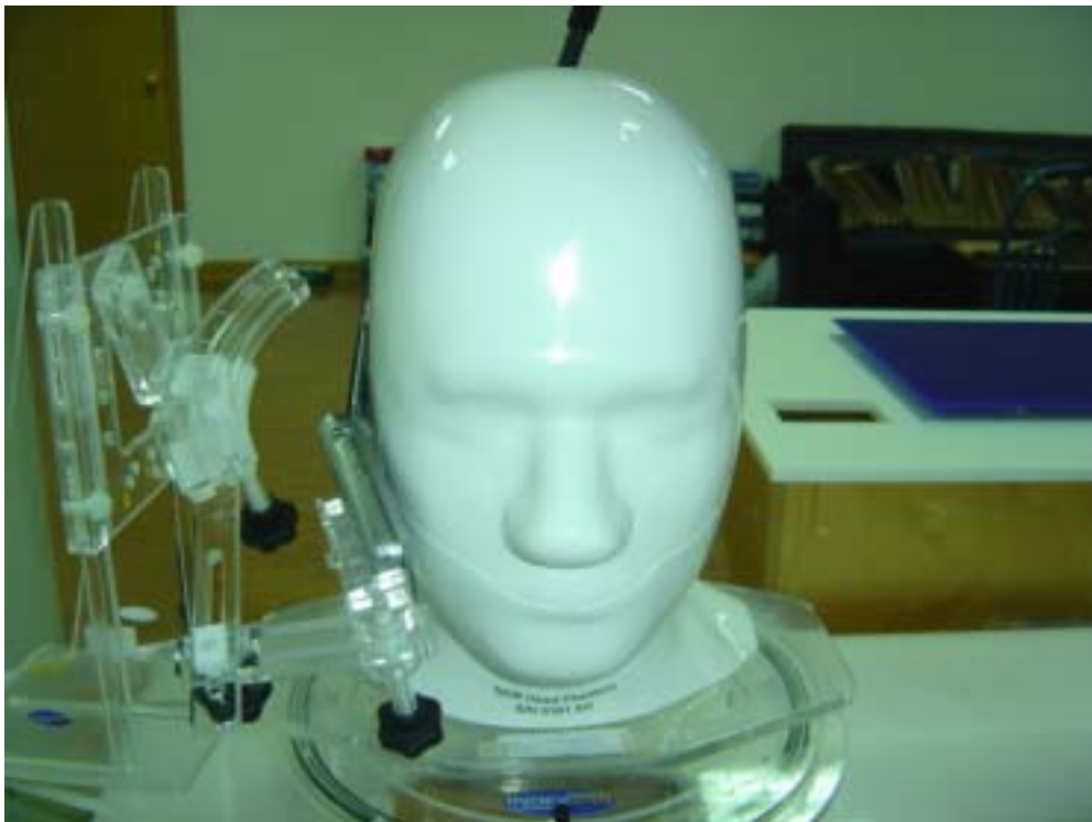
Fig.5 EUT Right Head Touch Cheek Position
