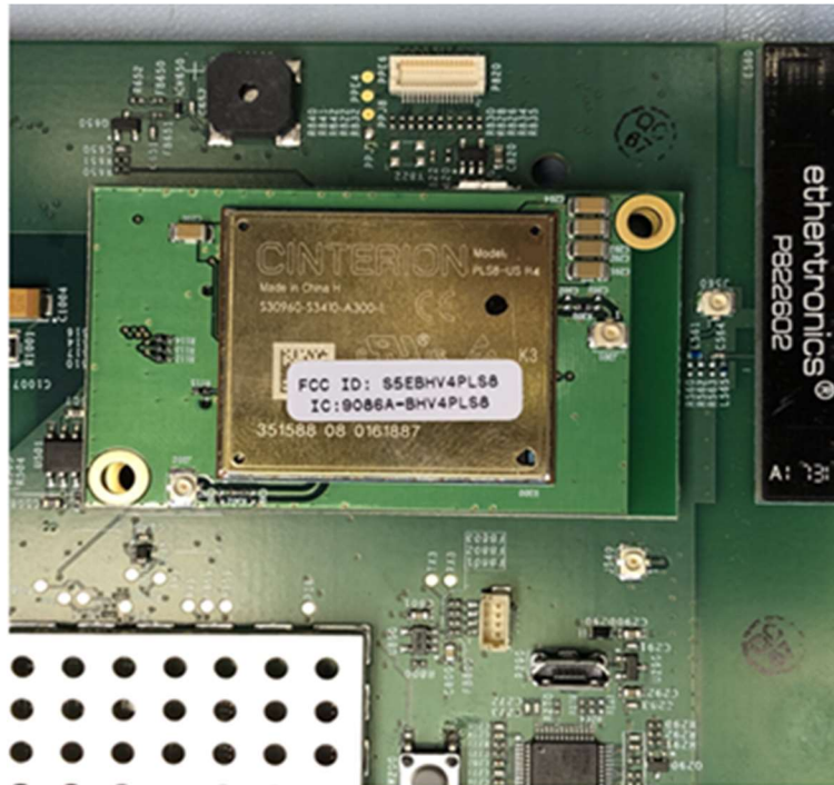
Satellite Tracking of People Modem Module board
