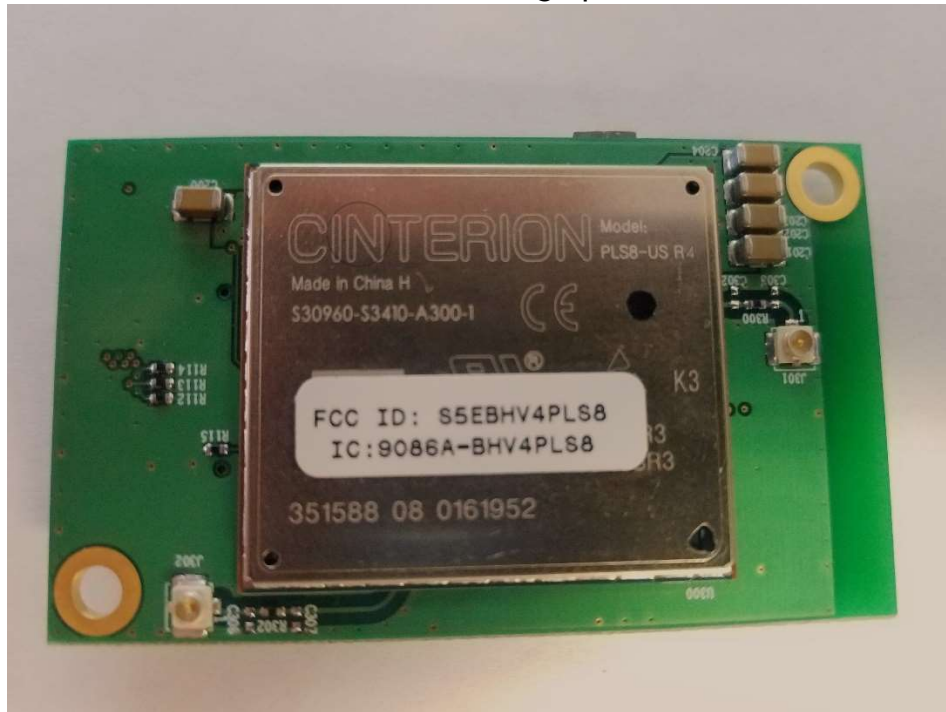
Satellite Tracking of People Modem Module board
