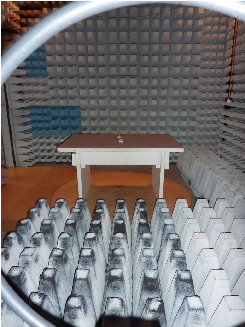
160125_i2.JPG: PERU_098, test setup fully anechoic chamber below 30 MHz
