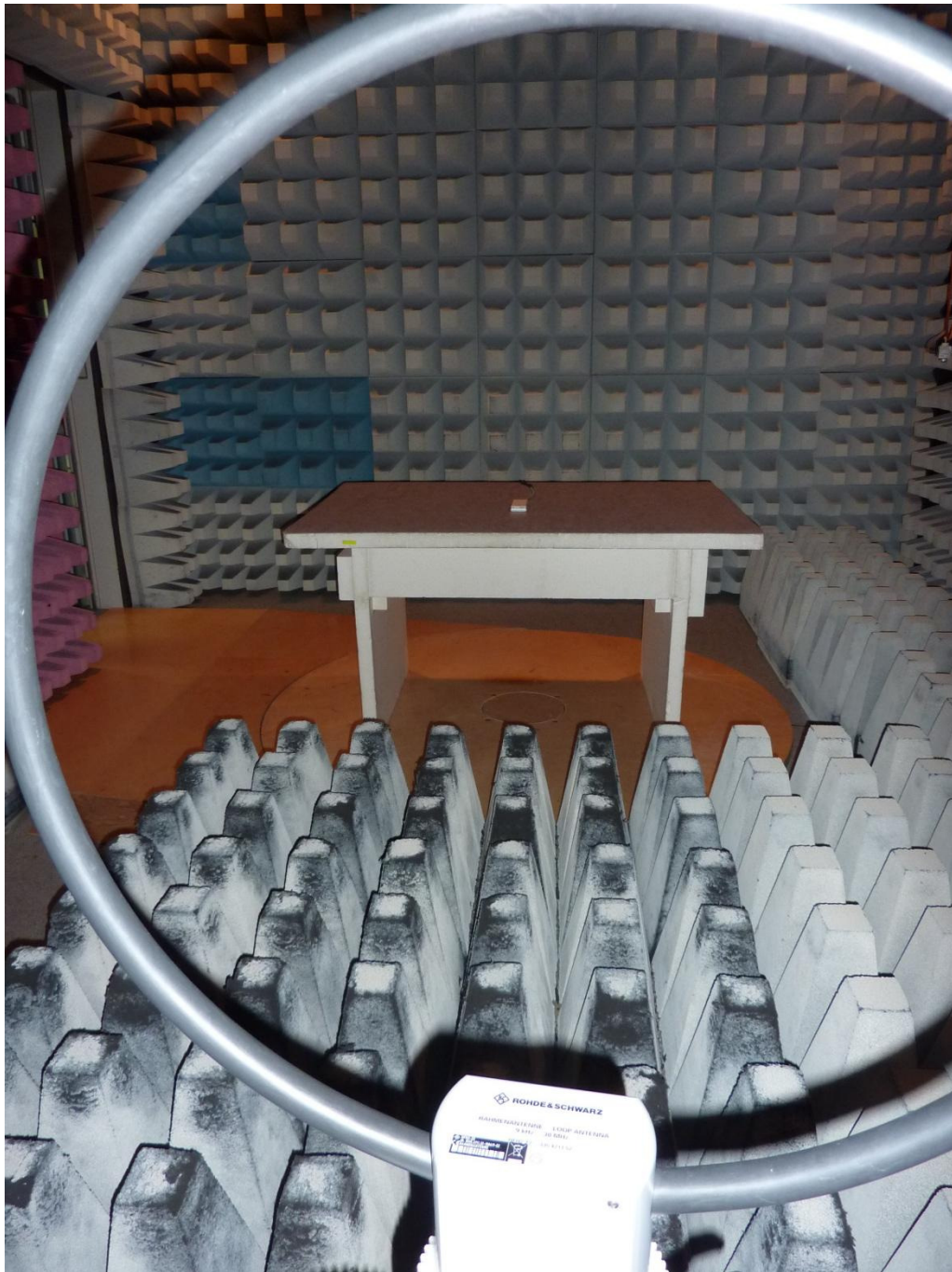
160125_i1.JPG: PPU_098, test setup fully anechoic chamber below 30 MHz
