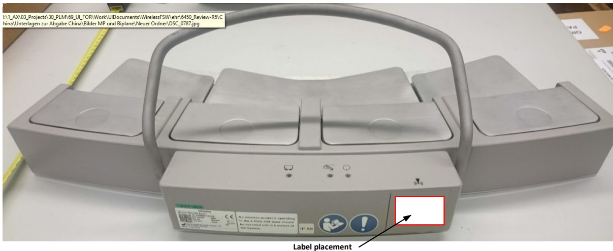
Figure 6: Label placement on Wireless XRay Footswitch Bilplane Model 04787805
