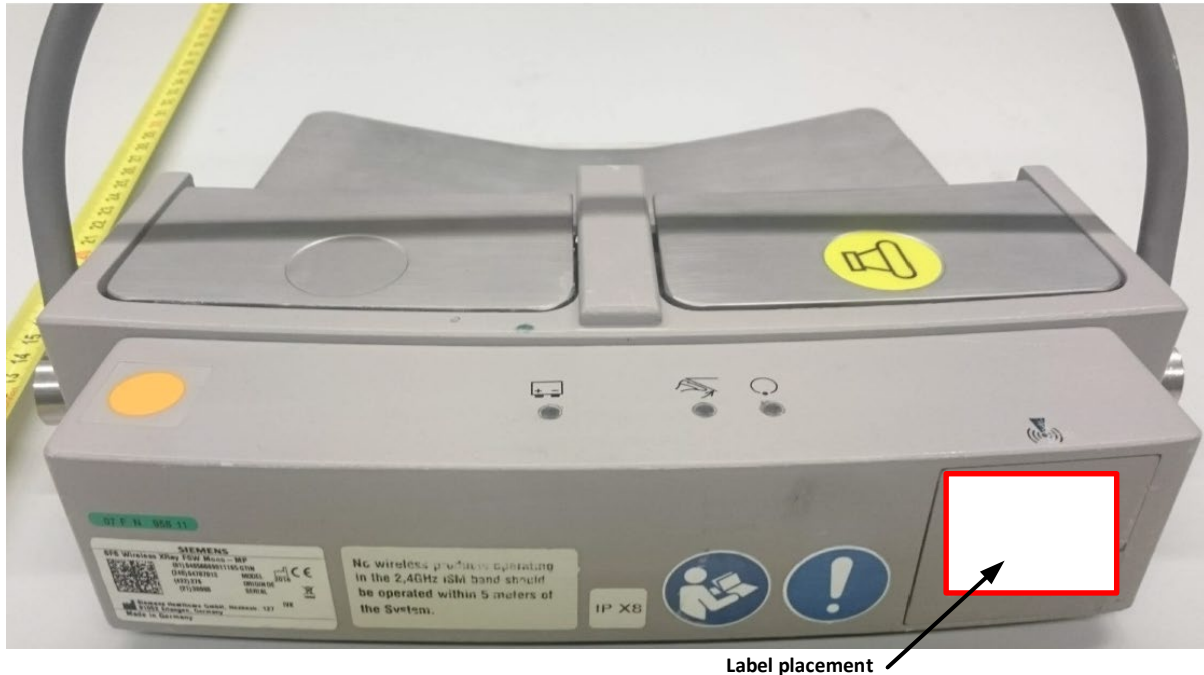
Figure 4 : Label placement on Wireless XRay Footswitch Mono-MP Model 04787813
