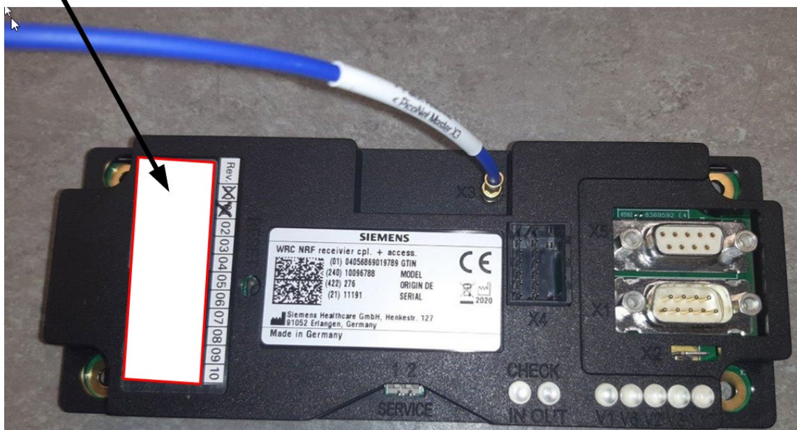
Figure 1: Label placement on WRC NRF receiver cpl. Model 10096788
