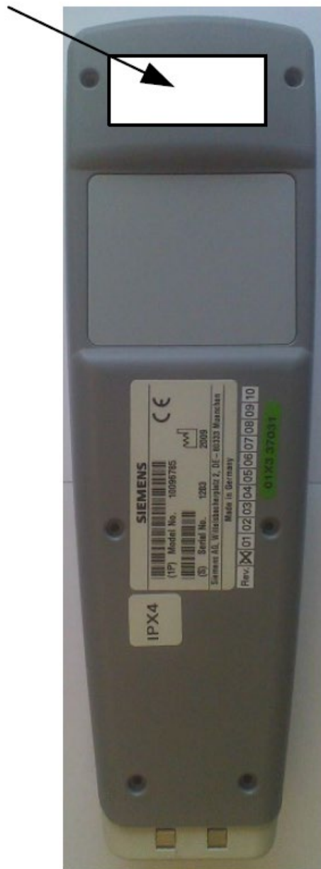
Figure 3: Label placement on Radio remote control WRC NRF Model 10096785
