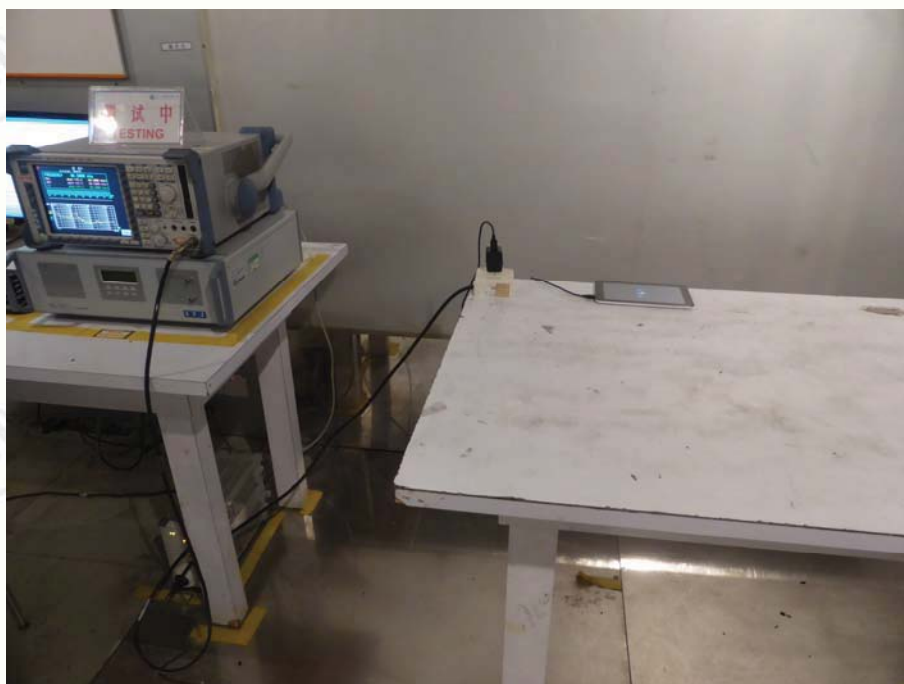
TEST SETUP OF CONDUCTED EMISSION
