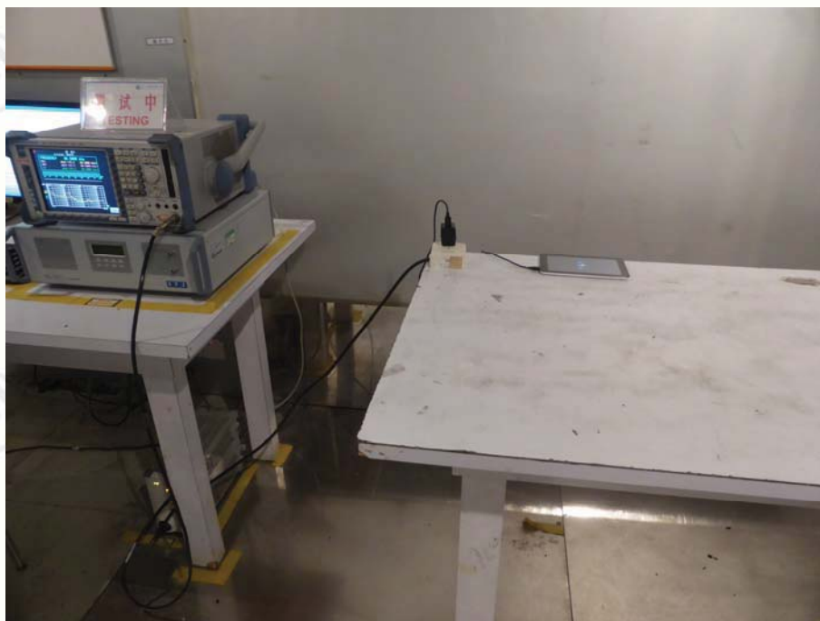
TEST SETUP OF CONDUCTED EMISSION
