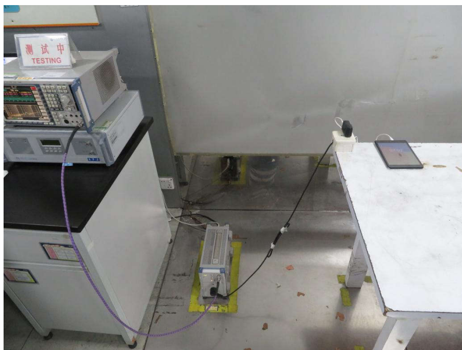
Conducted Emissions Test Setup
