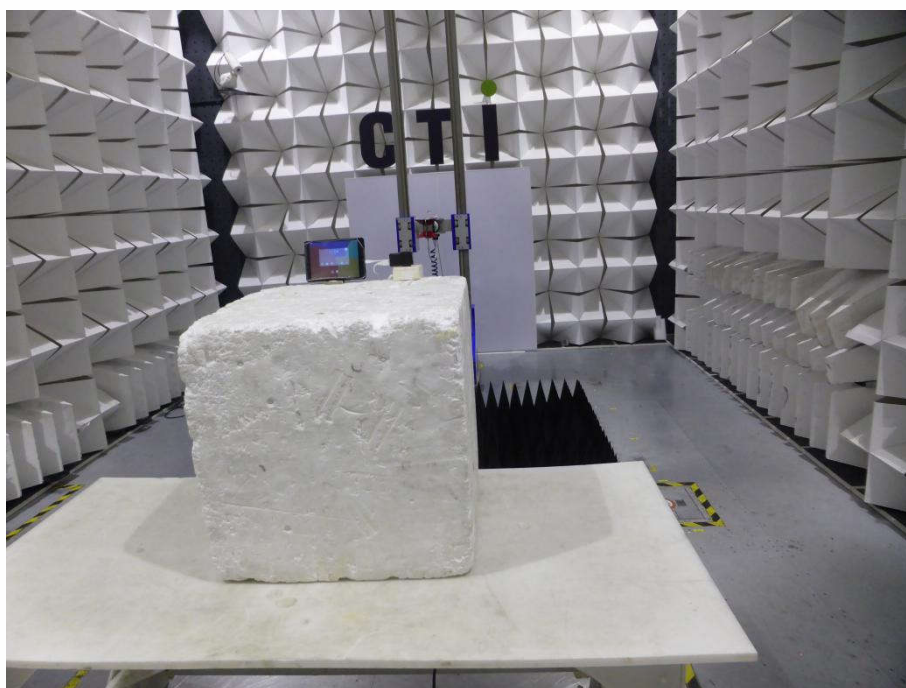
Radiated spurious emission Test Setup-2(Above 1GHz)
