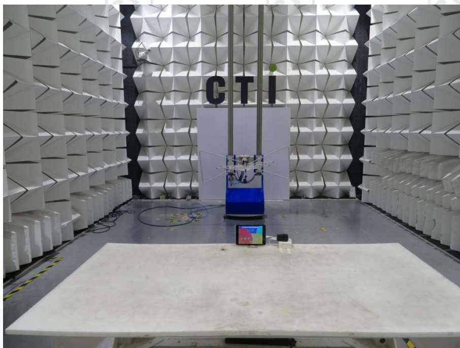
Radiated spurious emission Test Setup-1(Below 1GHz)
