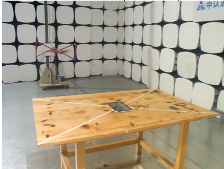
Radiated Emission (1GHz-25GHz)
