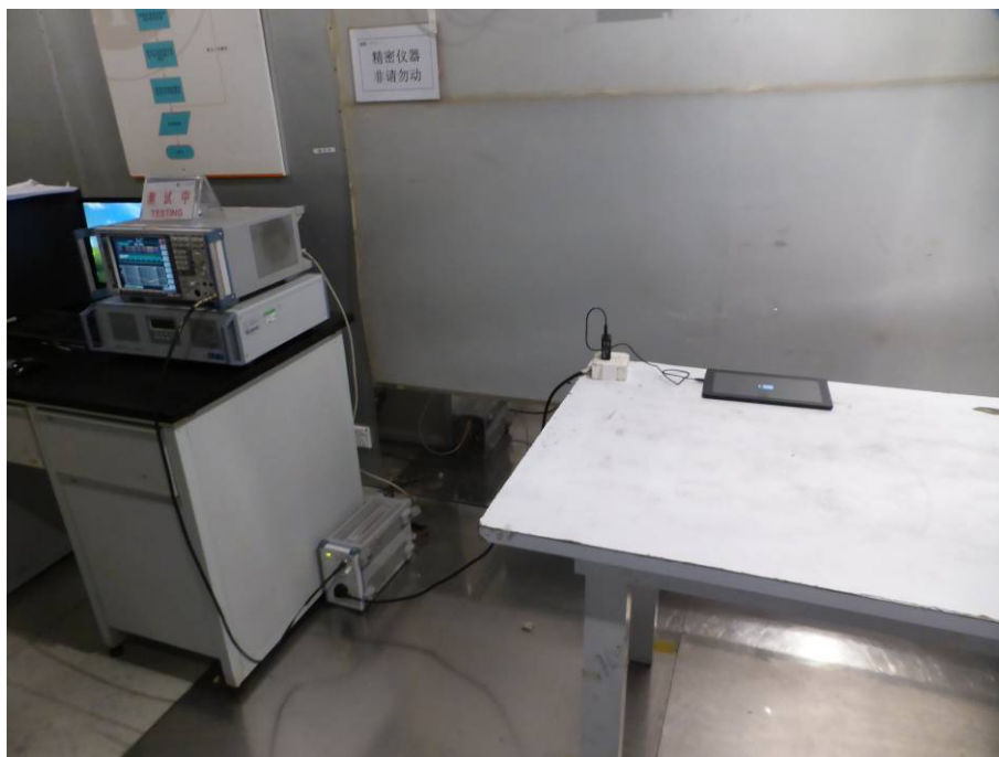
Conducted emission Test Setup
