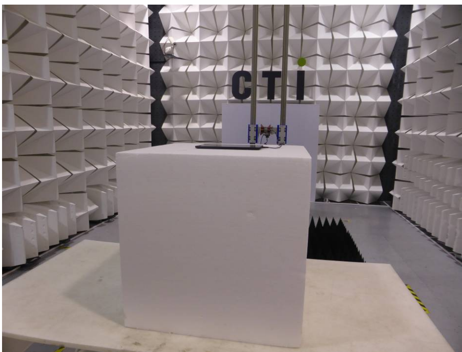
Radiated spurious emission Test Setup-2(Above 1GHz)
