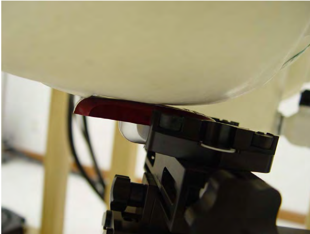
Fig.4 Right Hand Touch Cheek Position
