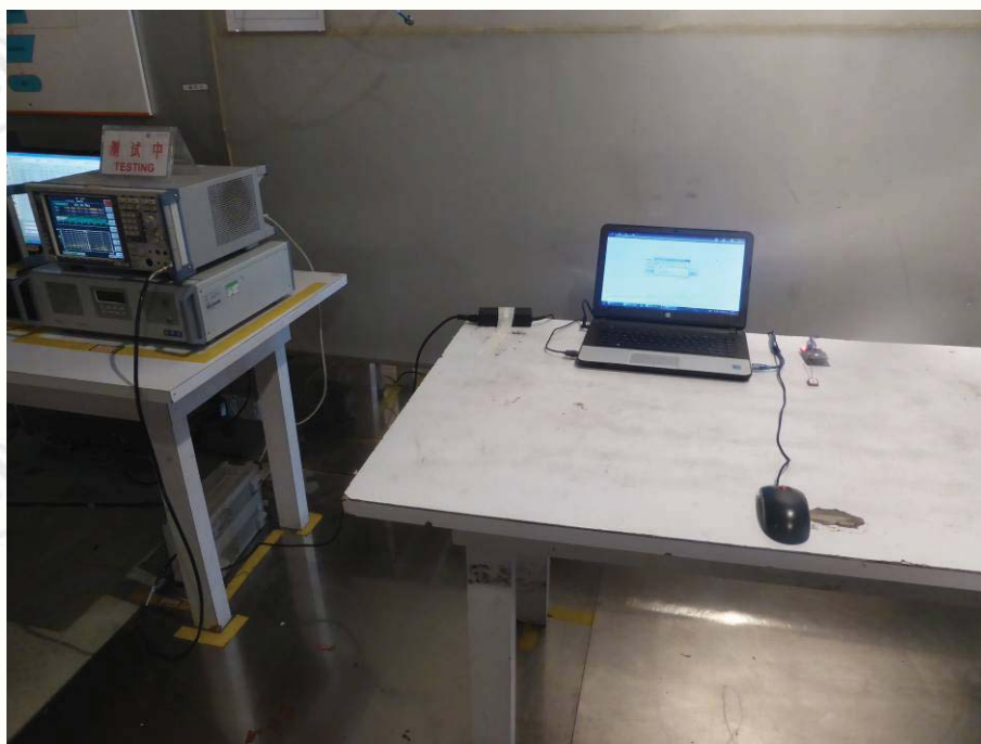
TEST SETUP OF CONDUCTED EMISSION
